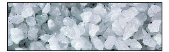
YETI Corundum is a iron-free material with a high level of whiteness, extreme hardness and with a large selection of precise grits.
