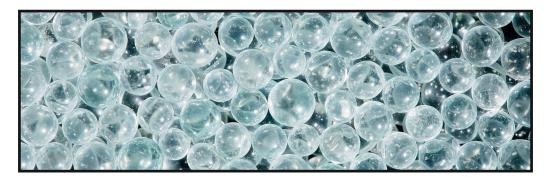
YETI Glass beads are a mineral, iron-free reusable blasting agent. Due to their round grain shape, they have a low abrasive effect and are therefore ideally suited for gentle cleaning/application. The highest value is placed on cleanliness in the production process. Available in 25 kg bag in the grain size 50 my.
